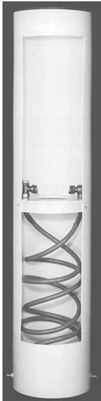
The MUELLER THERMAL-COIL Meter Box provides a means to allow a meter to be read and maintained even though it is set deep in the ground to resist freezing. The THERMAL-COIL Meter Box is designed with the meter installed on a platform that normally sets near the bottom of the box where the ground temperature keeps it warmer. The meter and platform are connected to the service line by coils of polybutylene tubing which allow the meter and platform to be raised to the surface.
