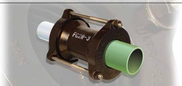
It may be small, but this robust 3" coupling offers a large range and is exceptional for connecting nominal size, dissimilar pipe. As with all our FC2W Ultra-Flex couplings, there is no disassembly required. It simply slides onto the end of the pipe, and as the fasteners are tightened with a deep-well socket, the gaskets compress firmly on the pipe.
