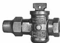
MUELLER MARK II ORISEAL Curb Valve Inlet: Copper flare nut Outlet: F.I.P. thread Quarter turn check
