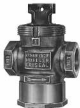
MUELLER ORISEAL Curb Valve F.I.P. thread - both ends Quarter turn check and Minneapolis top thread
